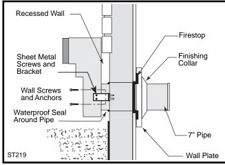
Fig. 31 Use extension brackets to mount snorkel against recessed wall.
